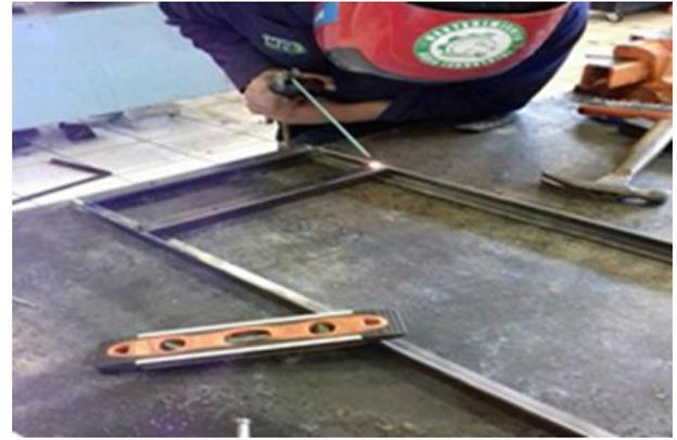
**Figura 3** Base de cold rolled
